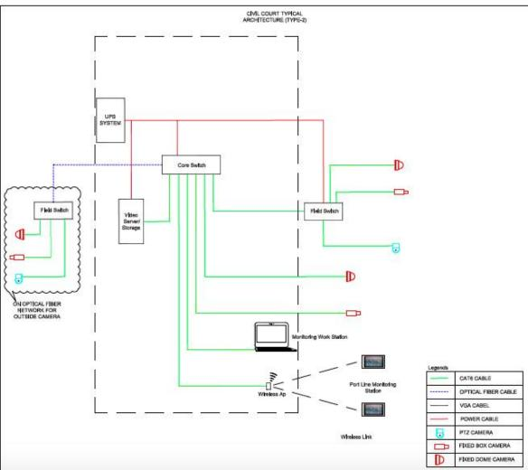
1. The surveillance solution considers use of high resolution fixed cameras. Good resolution cameras are considered for the situational cameras within the premises. All the entrance points within the buildings have high resolution cameras considered for clear identification of the persons entering and leaving the building.
